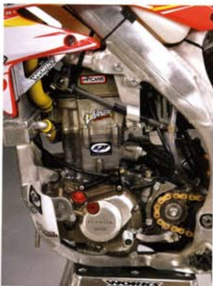
Between the stroker crank, the Hot Cams Stage Two cam and the Varner headwork, the CRF471 was incredibly fast.
